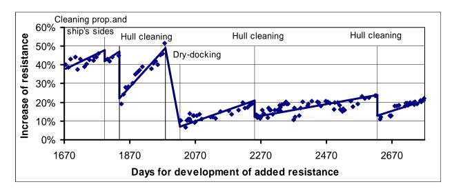
2. This ship (below) came out from the dry-dock with a remarkably high added resistance (40%), and this resistance was constant for a period, until it suddenly dropped. After this the added resistance developed very fast (6% per month). A hull cleaning removed approximately half of the added resistance, but the resistance is developing fast again after the cleaning. It is a clear example of a poor treatment in the dry-dock.
