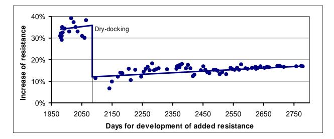
2. Example (below) of a more pronounced development of the added resistance. Here, the propeller polishing at 6 month intervals resulted in a 5 ton per day fuel saving and the hull cleaning resulted in approximately 10 tons per day fuel saving. The development of resistance of the hull and propeller is 0.7 - 1% per month.
