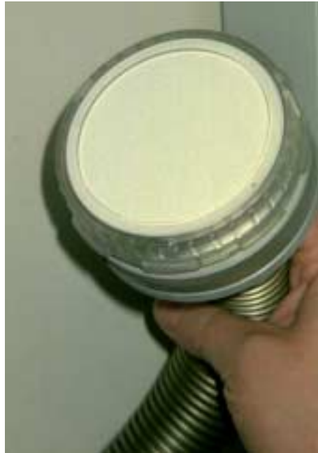
Figure 11. A gelatine membrane filter unit used in the MD8 filtration equipment.
