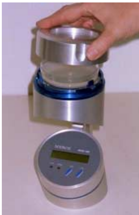
Figure 7. The MAS-100 air sampler is an impactor.
