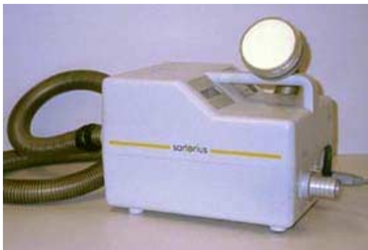
Figure 10. The MD8 equipment is based on the air filtration technique.
